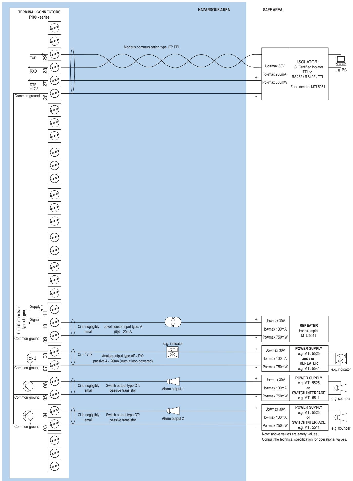
Configuration example IIB / IIIC and IIC - F173-A-AP-(CT)-OT-PD-XI - Power requirement 16 - 30V DC
