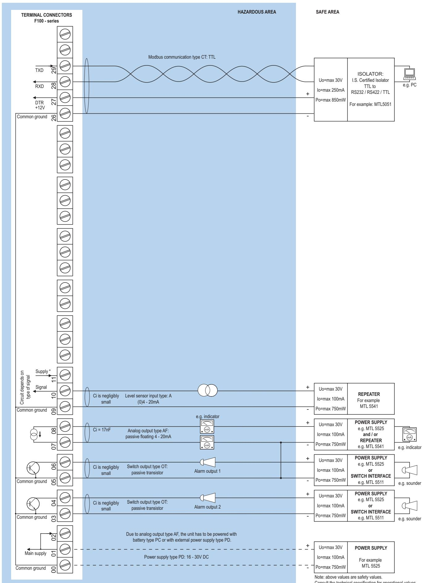
\* Note power supply type PD: the supply voltage to the analog sensor is as connected to terminal 1 (internally linked).
