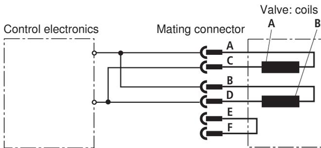
The coils are connected in parallel in the mating connector or on the amplifier (see figure).
