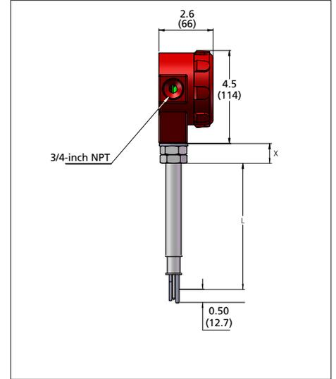
Remote Probe VTP—Front View
