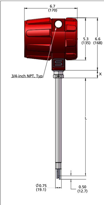
P2-DD Flange Fitting—Side View
