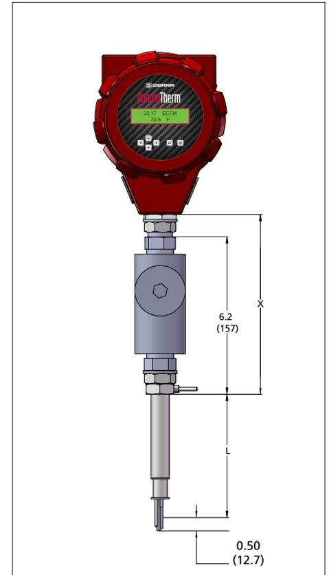
Note: All dimensions in inches with (mm) in brackets; certified drawings available upon request. All drawings have  $\pm .25$  inch (6.4 mm) tolerance.
