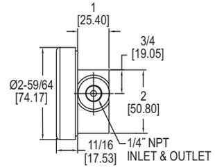
The **Series DTFW Variable-Area Flowmeters** for Liquids and Oils measure water or oil flow rates with  $\pm 2\%$  of full-scale accuracy at a competitive price. Available in 1/4", 1/2" and 1" connections for a wide variety of applications and comes calibrated for horizontal in line mounting.
