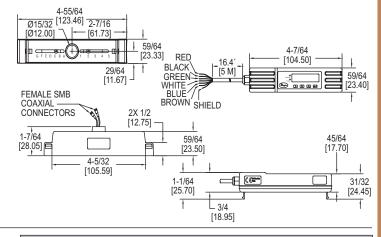
The Model UFM Compact Ultrasonic Flowmeters are economical, clamp-on, ultrasonic flowmeter. The Model UFM implements the transit-time difference to measure flow rates in pipes and can measure velocity and flow in pipes with outside diameters ranging from 0.98 to 4.62" (24.89 to 117.35 mm). This model comes with a volume pulse and 4-20 mA flow rate output.
