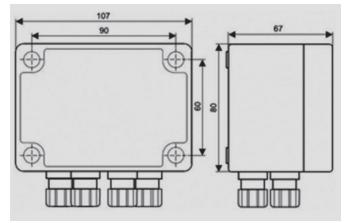
The level limit controller TS-KGS-W1222 is designed for the evaluation of 2-wire or 3-wire level limit switches. For 2-wire level limit switches with additional programming wire, such as TS-KGS, a special design for simplified sensor configuration is available.
