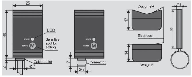
**Design SR** is fixed on the non-conductive sight tube ( $\emptyset$  15 up to 50 mm) by plastic straps **Design F** is installed with a self adhesive layer directly on the flat vessel surface.
