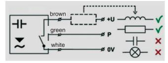
Sensor supply: **+U** connected on brown conductor, an electrical load (e. g. relay) gets interposed. **0V** connected on white conductor. **Programming wire** "**P**" (green) is used for configuration. The sensor output is equipped with short circuit protection. Capacitive loads or low resistance (e. g. bulb) is evaluated by the sensor as short circuit.
