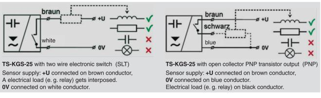
The sensor output is equipped with short circuit protection. Capacitive loads or low resistance (e. g. bulb) is evaluated by the sensor as short circuit.
