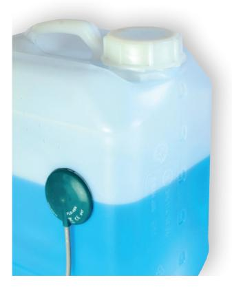
The capacitive level limit switch **TS-KGS** is designed to monitor level limits of liquids in nonconductive plastic or glass vessels. The flexible polyurethane-housing is mounted with self adhesive layer directly on the vessel. The sensor has to be mounted on the height of the level limit which is to be monitored. The maximum possible thickness of the vessel wall is depending on the permittivity  $\varepsilon_r$  (dielectric conductivity) of the filling medium.
